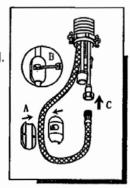
4. Proper installation of the hose weight kit will insure that the hand spray retracts smoothly. On the handspray side of the hose, measure 15" down from the body of the faucet. Install the hose weight kit at this point. Pull out on the handspray. It should move easily and retract smoothly. Reposition the hose weight kit as necessary. Make sure that the hot and cold supply hoses do not interfere with the handspray hose. They can be repositioned slightly if necessary.
