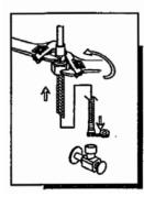
5. Attach water supply hose to the faucet. To avoid breaking the copper tube from the faucet, usee two wrenched (as shown) to keep from the faucet when you tighten the nut, and attach the other end to the water supply.
