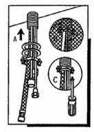
3. Re-assemble the mounting hardware onto the shank, use philips screwdriver for final tightening after spout is aligned.
